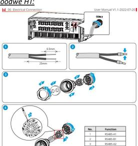
Using COM2 port on inverter. RS 485 pin 2 > SEC COM B RS 485 pin 1 > SEC COM A
