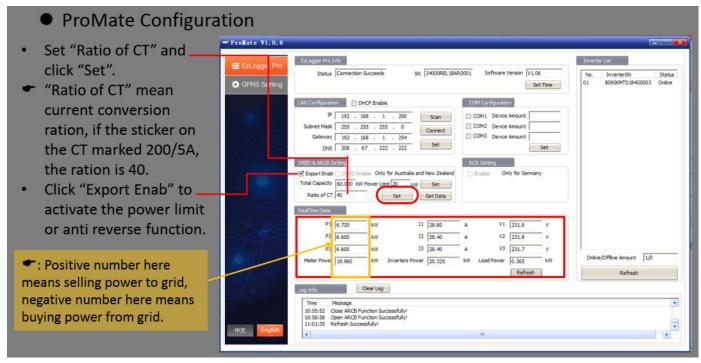
From real time data under this scenario, the P1, P2 n P3 should be negative and I1, I2 n I3 should be negative as well. Inverter should be 0kW.
